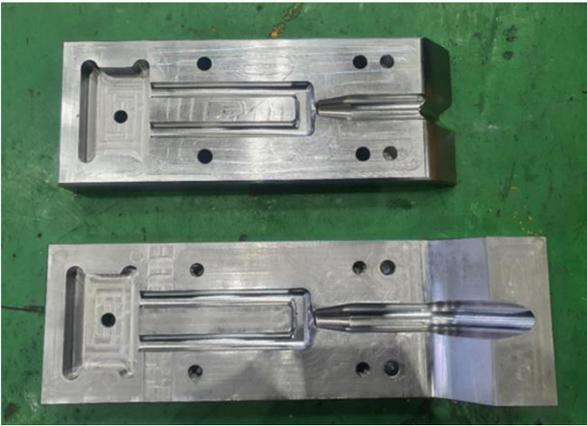
Fig. 3. SKD61 steel salt core mold.
